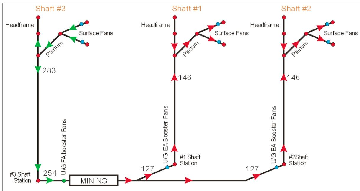
Figure 1. Future overall mine flow distribution.
