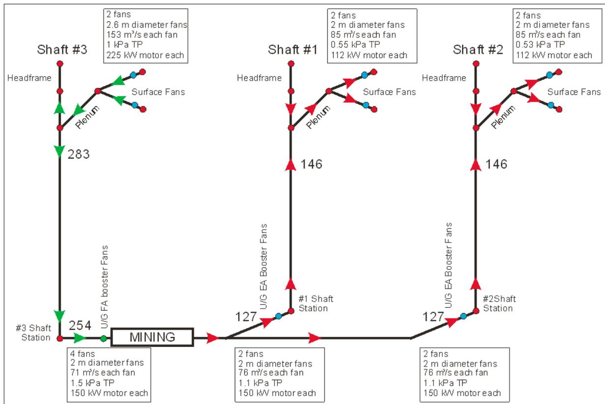
Figure 2. Mine primary and main booster fan requirements.
