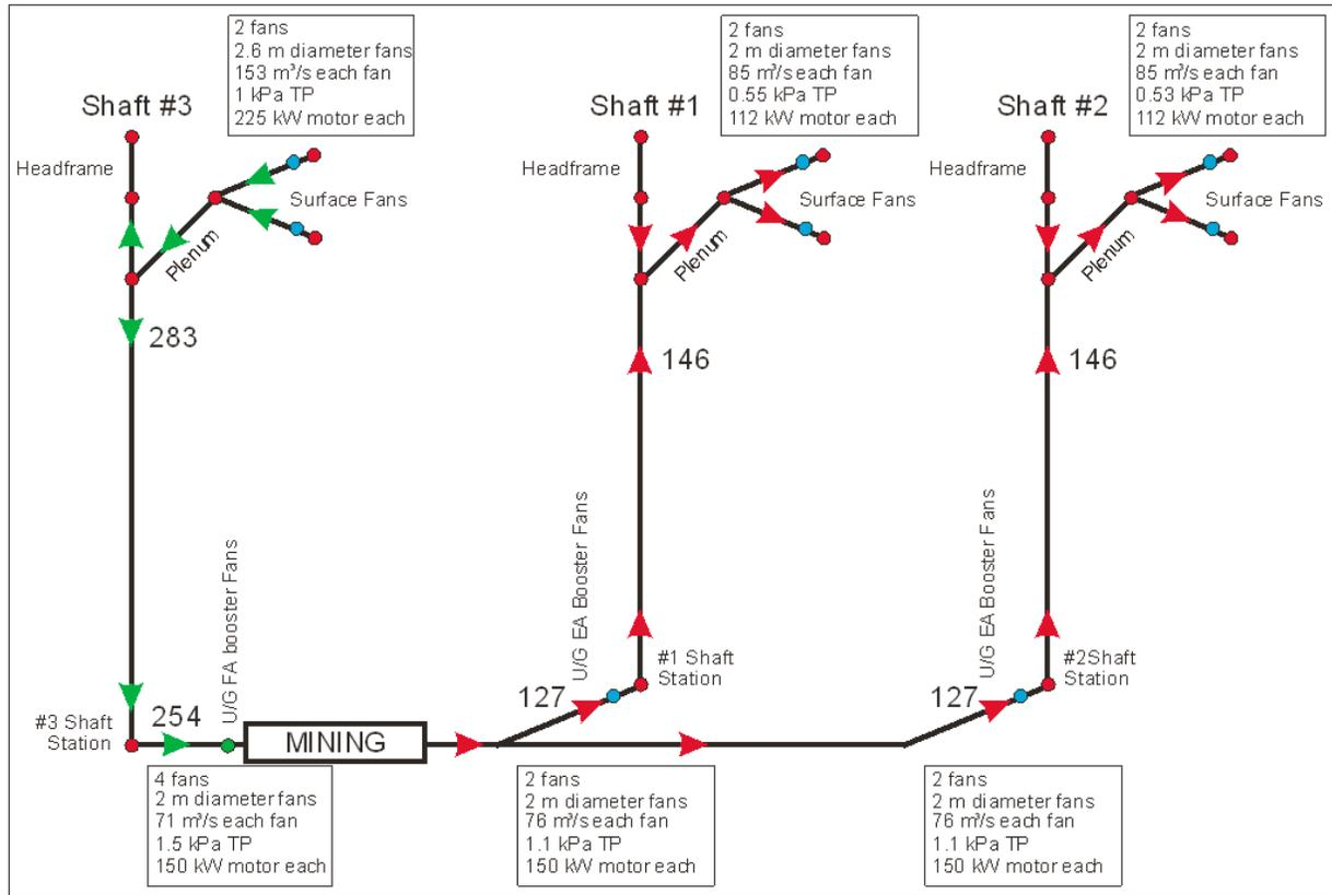
Figure 1: Mine primary and main booster fan requirements [1]
