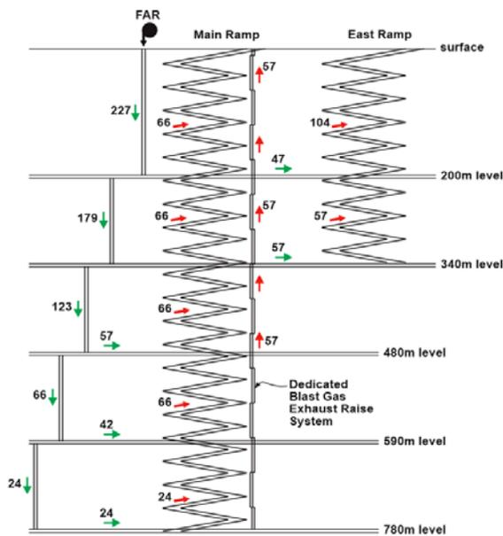
Figure 4. Modified Mine Ventilation Network Schematic (flows in m<sup>3</sup>/s).
