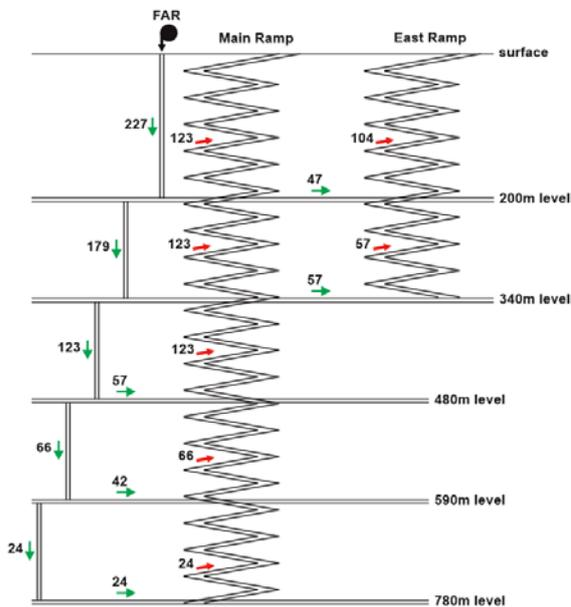
Figure 3. Original Mine Ventilation Network Schematic (flows in  $\text{m}^3/\text{s}$ ).
