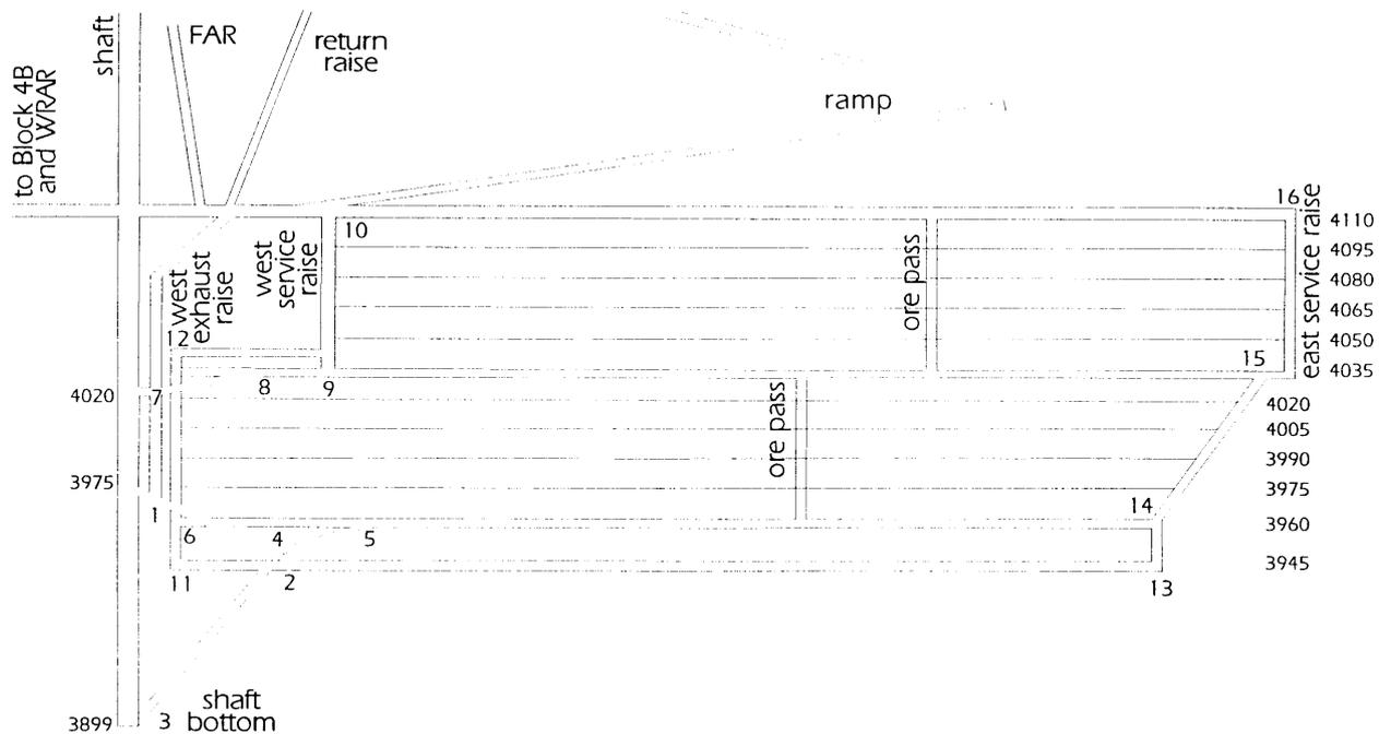
Figure 3. Schematic of development stages for Block 5
