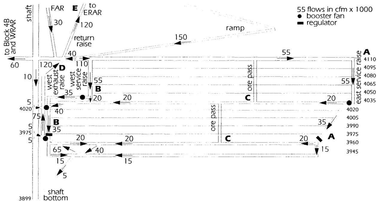
Figure 2. Schematic of Block 5 ventilation system
