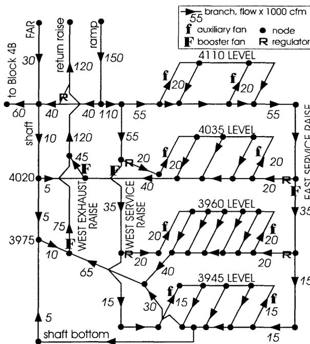
Figure 4. Ventilation circuit for Block 5
