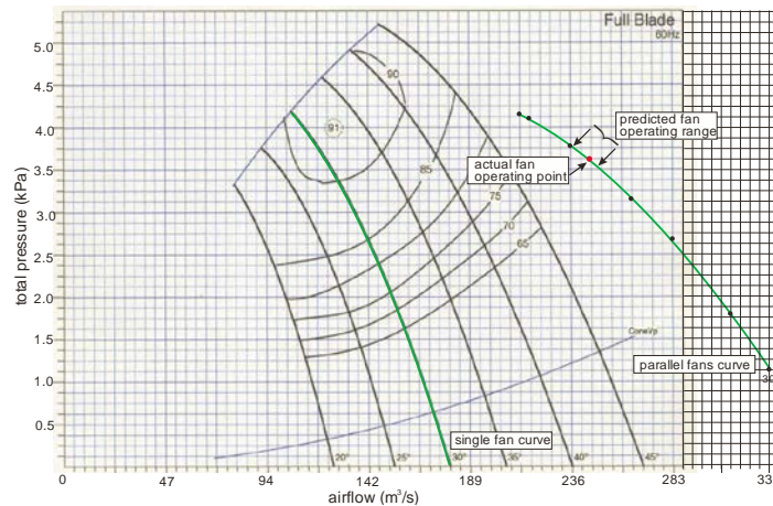
Figure 10 - Parallel fan operation @ 30° (De Souza, 2012)
