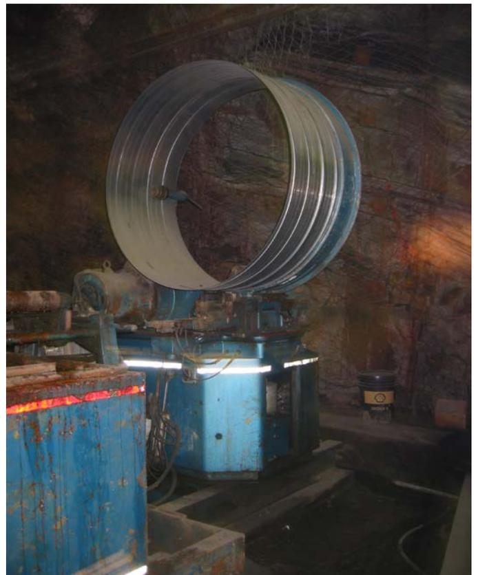
Figure 7. Underground manufacturing of rigid tubing.
