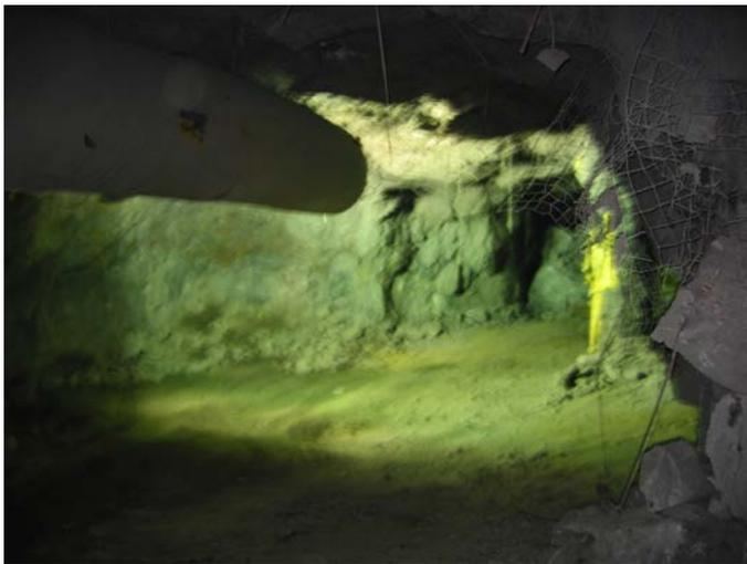
Figure 2. The end of the ventilation column is positioned at the centre of the drift and high at the back to provide adequate dilution of contaminants.
