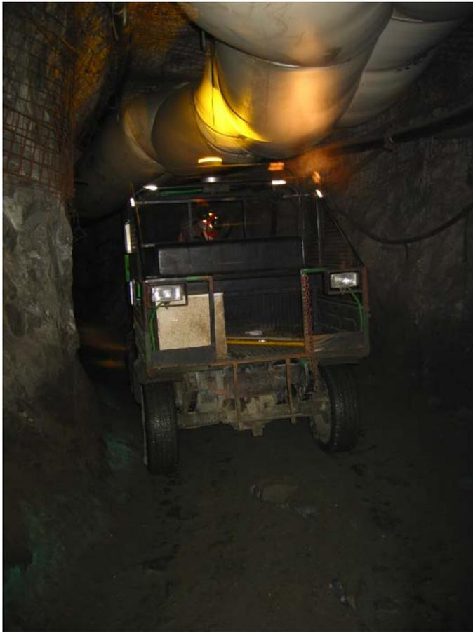
Figure 5. Sufficient clearance between ducting and mobile equipment should be provided to prevent damage to column.
