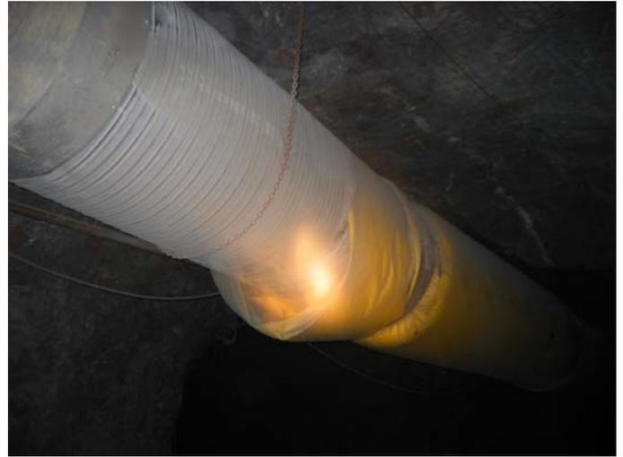
Figure 6. Flexible and rigid tubing used in the same column.
