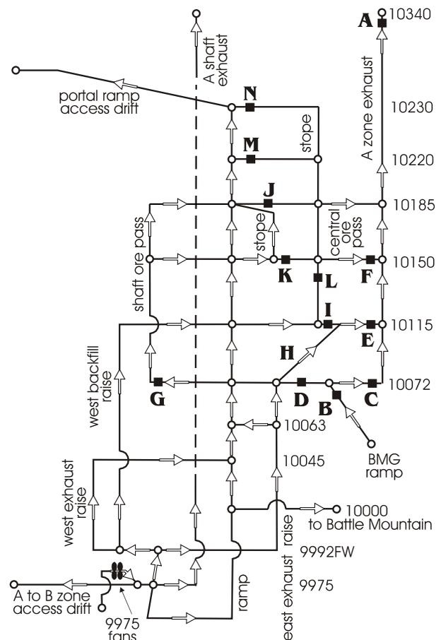
Figure 3. Underground stations modified during preliminary simulations
