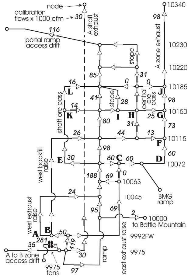
Figure 2. Ventilation circuit for the Williams 'A' zone exhaust system
