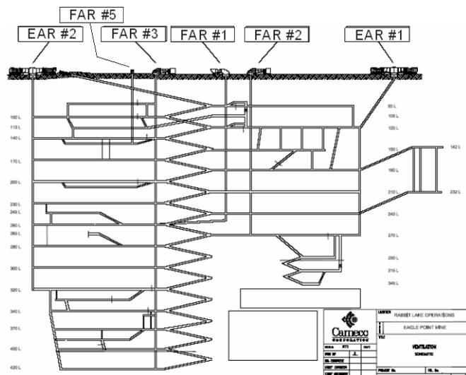
Figure 1. Rabbit Lake ventilation system schematic
