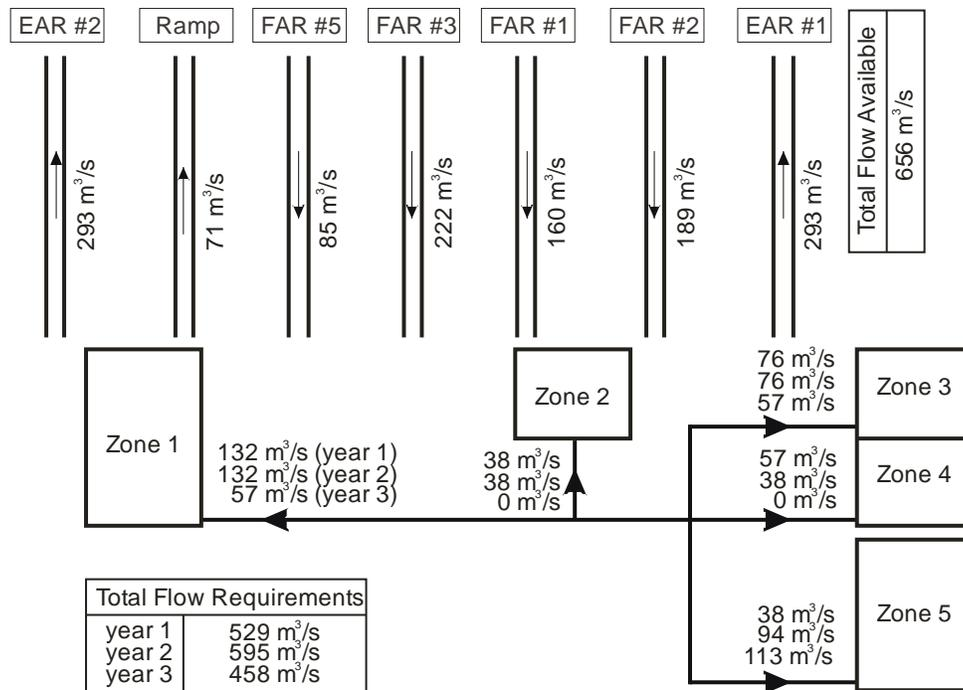
Figure 2. General ventilation schematic with required and available airflows
