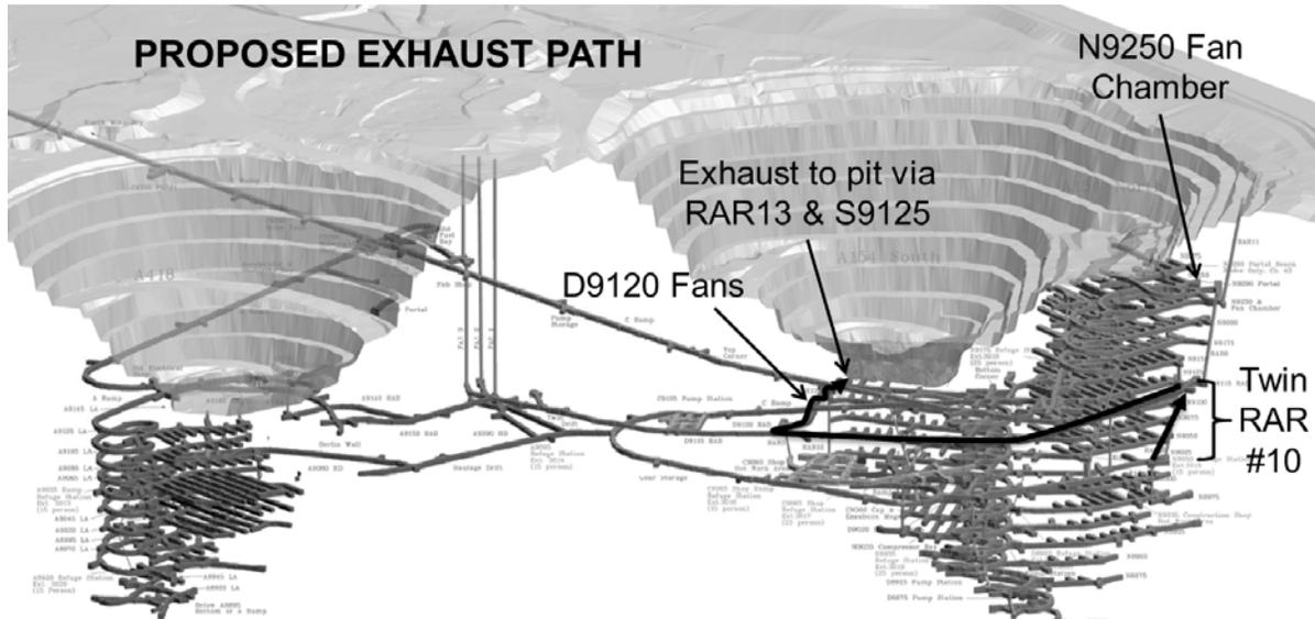
**Figure 5. Isometric view of Diavik Underground with proposed exhaust path highlighted through the RAD and RAR #10 Twin**
