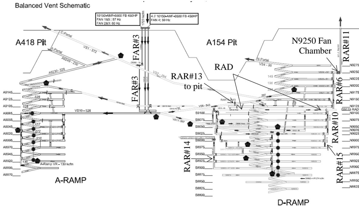
**Figure 4. Diavik ventilation Schematic with infrastructure tested for expanded capacity identified**
