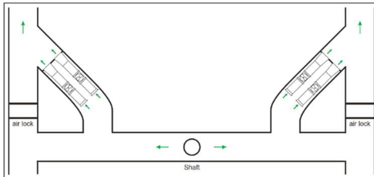
Figure 3. Booster fan installation schematic (AirFinders Inc., 2013)
