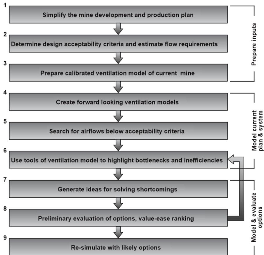
Figure 1. Methodology for booster fan sizing and selection
