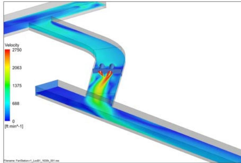
Figure 5. Optimized booster fan installation siting
