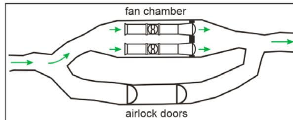
Figure 2. Booster fan installation schematic
