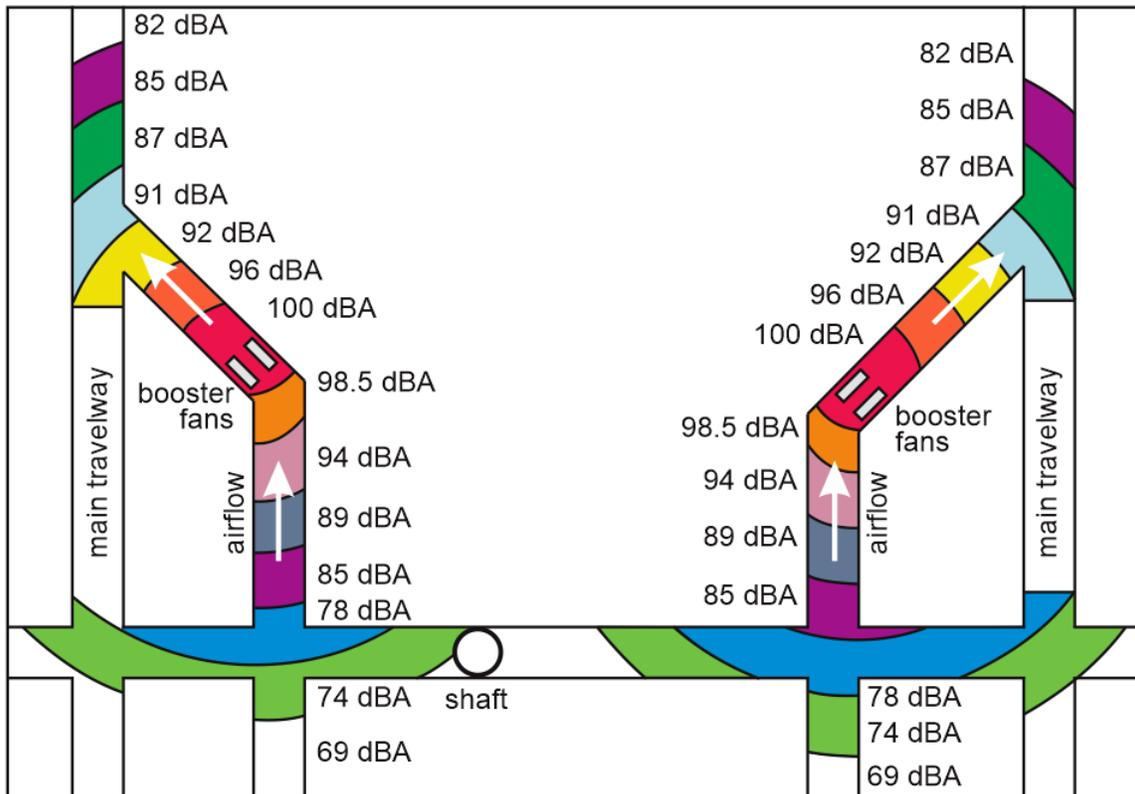
Figure 6. Estimated dBA contour map at the shaft area
