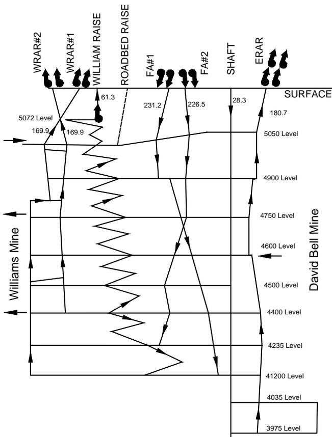
Figure 2. Caption of the mine main ventilation system, including the effects of the Williams fan. Airflows in  $\text{m}^3/\text{s}$ .
