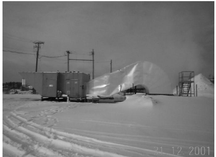
The above implementations resulted in the desired reversal of the airflow in the mine shaft. The mine shaft started to upcast at a rate of 14.2 m<sup>3</sup>/s. A schematic of the achieved flow distribution at the upper section of the mine is shown in Figure 8.
