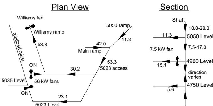
Figure 3. Caption of original airflow distribution in the upper part of the mine before the test. Airflows in  $\text{m}^3/\text{s}$
