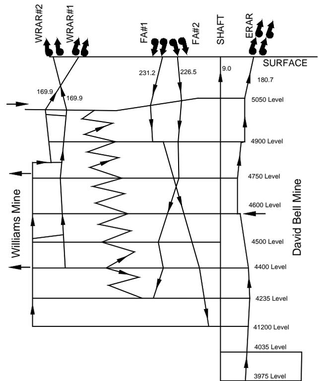
Figure 1. Caption of the original mine main ventilation system. Airflows in m<sup>3</sup>/s.
