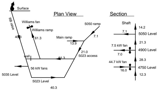
Figure 8. Caption of the airflow in the upper part of the mine following the implementations from section 6. Airflows in  $\text{m}^3/\text{s}$ .
