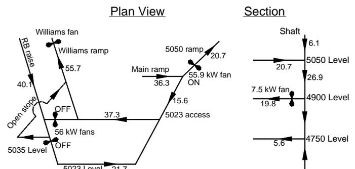
Figure 4. Caption of airflow distribution in the upper part of the mine during the test trial. Airflows in  $\text{m}^3/\text{s}$
